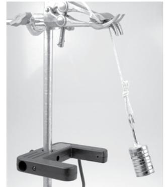
The diagram above shows how Time Machine measures SHM:-
