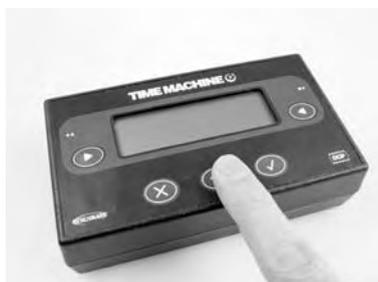
Switch on Time Machine and select 'Acceleration' followed by the input the light gate is connected to. Select the picket fence and enter the gap indicated on screen followed by the number of pickets.
