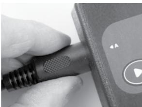
To use a light gate to control the start and stop of the stopwatch, connect a light gate to input 'A' and a light gate to input 'B'. An object passing through each light gate will start and stop the stopwatch respectively. You can also use a single light gate to start or stop a timing event and use the facia buttons to stop, reset or start depending on the input used.
