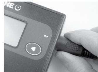
Mount the light gate into a stand or similar and place it such that the model car passes cleanly under the gate. Place a small interrupt card onto the model car to act as the trigger for the lap timer and adjust the height of the light gate so that the card triggers the gate.
