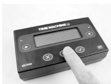
Switch on Time Machine and select 'Speed' then 'measure speed from A to B'. Enter the distance between the sound switches.
